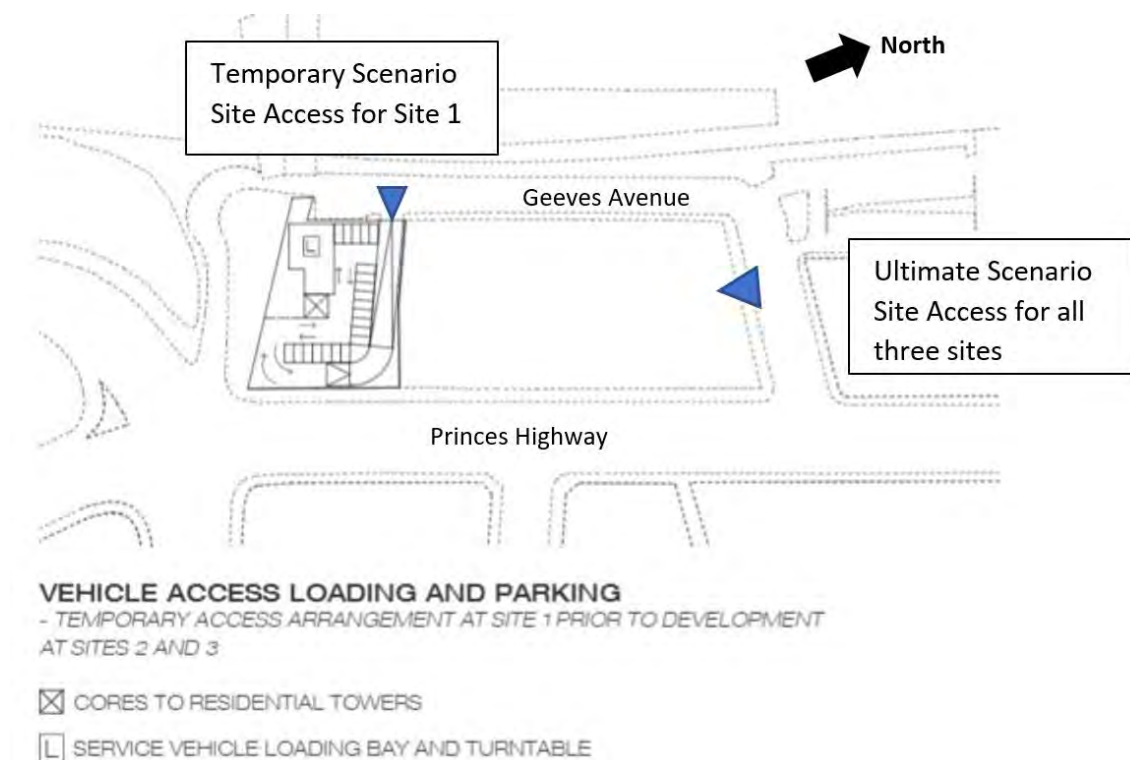
Figure 5.1: Site Access – Temporary and Ultimate Scenarios
